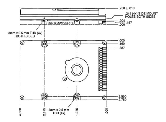
Figure 3. Mounting Configuration
