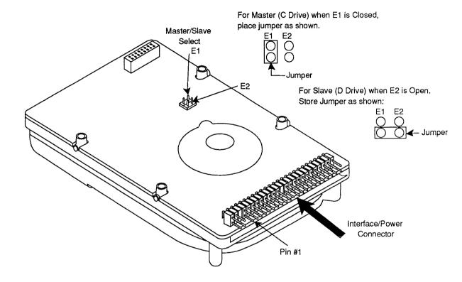
Figure 1. Master/Slave Jumper Configuration
